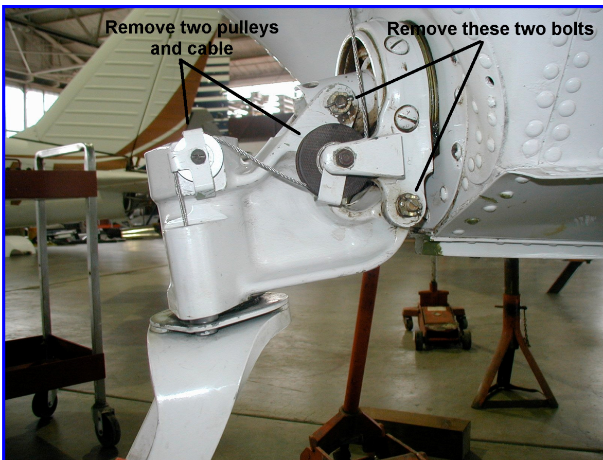
Tail wheel mechanism
