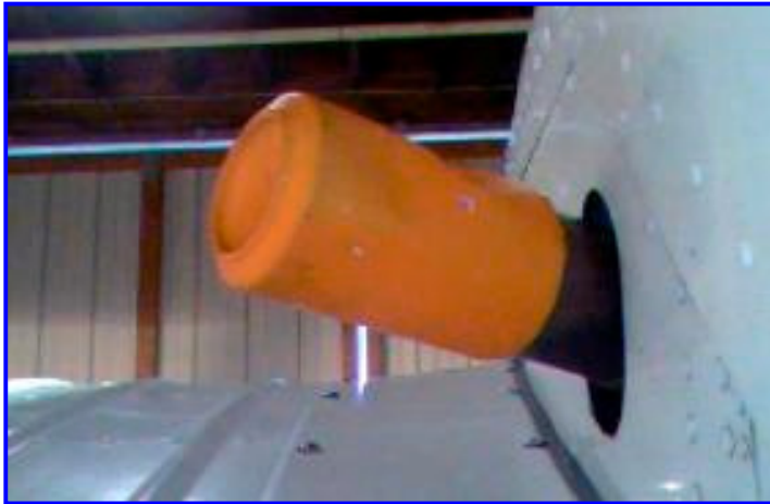
Can installed over exhaust pipe. Orange paint helps removal.
