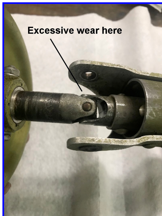
U-Joint on the forward end of control column
