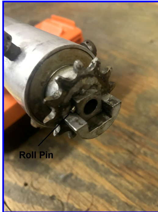
Torque tube end with sprocket. Note 1/16" roll pin.
