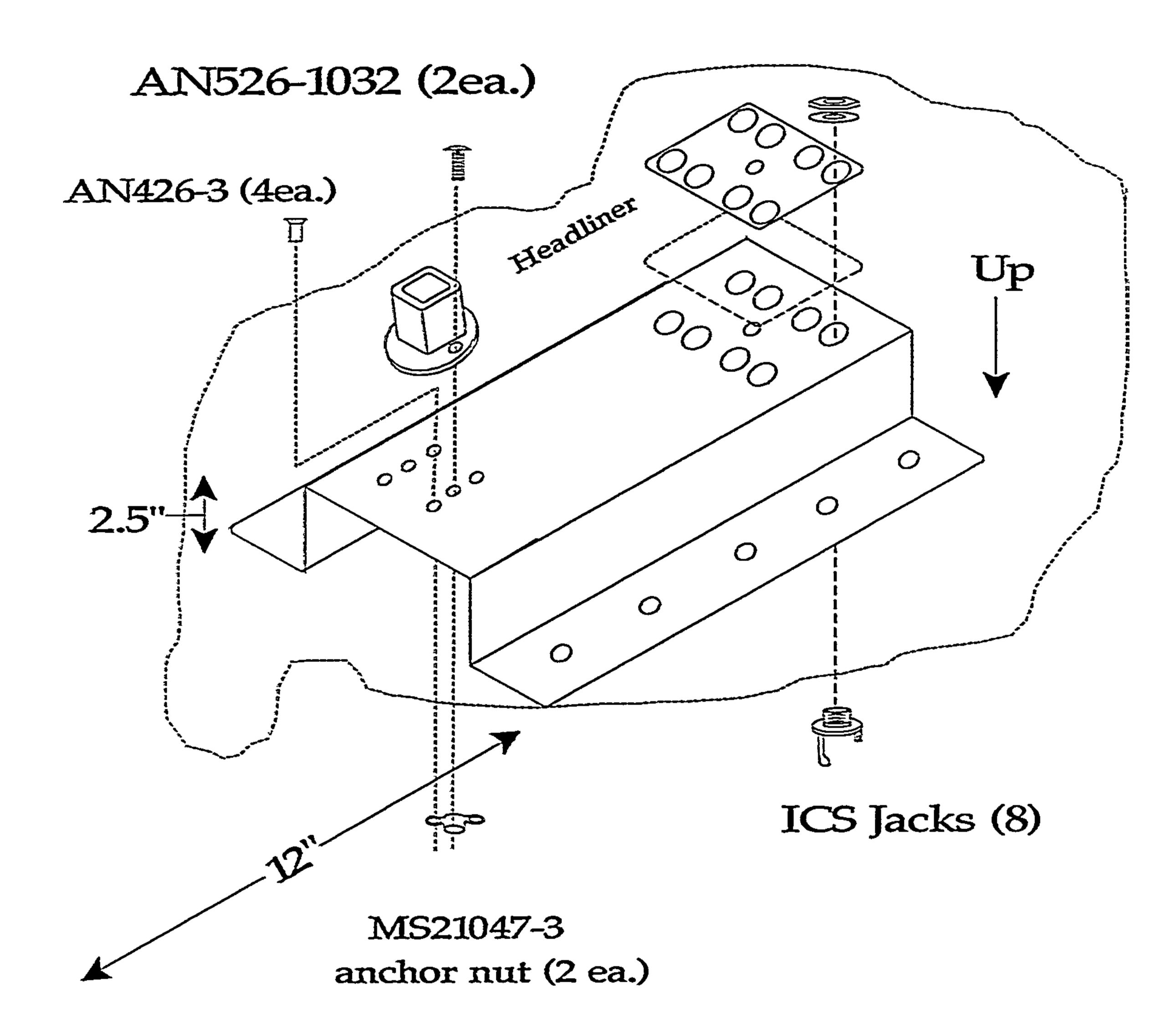
material - 2024 T3 aluminum .050 sheet rivets - AN426 4-4
