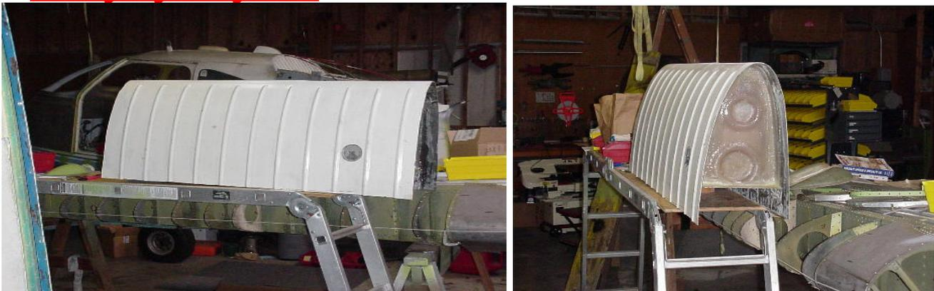
Second generation Seabee Guru, Henry Ruzakowski, has developed tanks that will hold a least 15 useable gallons per side. They are made of carbon fiber and kevelar and will gravity feed to the main tank with the operation of one lever. They will be done on a field approval, so you'll have to take your airplane to him in Florida. **So, let's plan a trip to Sun and Fun!!!** Call or email Henry for more information. 561-436-0821 [amphibs1@aol.com](mailto:amphibs1@aol.com)
