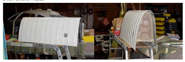
Second generation Seabee Guru, Henry Ruzakowski, has developed some <u>leading edge wing tanks</u> that will hold a least 15 useable gallons per side. They are made of carbon fiber and kevelar and will gravity feed to the main tank with the operation of one lever.
