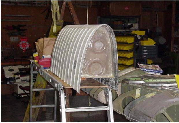
Second generation Seabee Guru, Henry Ruzakowski, has developed some leading edge wing tanks that will hold a least 15 useable gallons per side. They are made of carbon fiber and kevelar and will gravity feed to the main tank with the operation of one lever. They will be done on a field approval, so you'll have to take your airplane to him in Florida. **So, let's plan a trip to Sun and Fun!!!** Call or email Henry for more information. 561-436-0821 [amphibs1@aol.com](mailto:amphibs1@aol.com)
